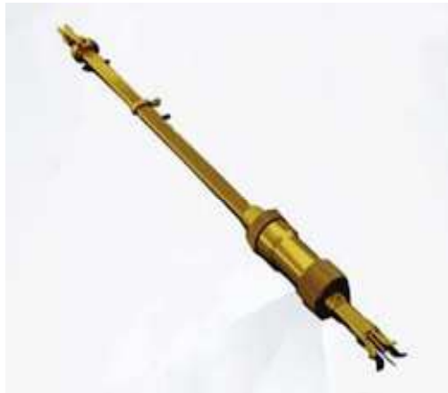
Modified Cole type Pitot tube with a safety pin in between the tips.
