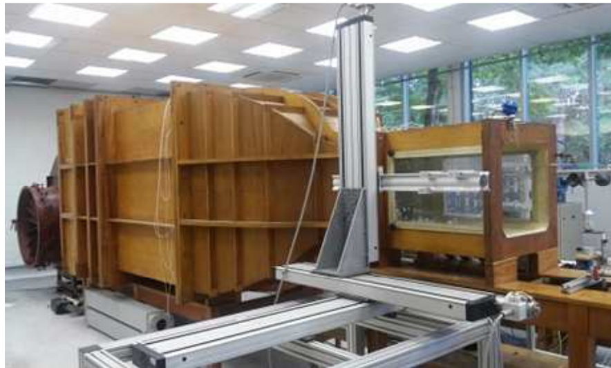
IPT aerodynamic wind tunnel (test section of 0.5 m x 0.5 m)
