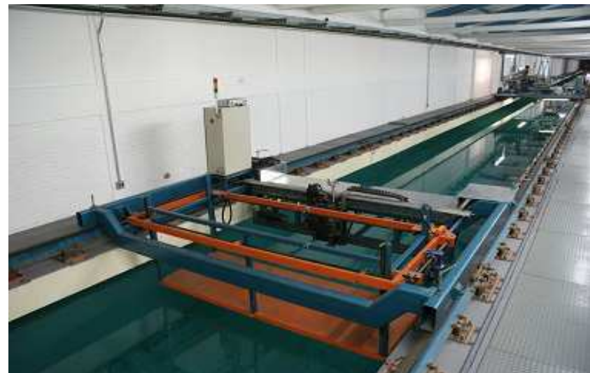
IPT Towing tank with 280 m long x 6.6 m width x 4.0 m depth
