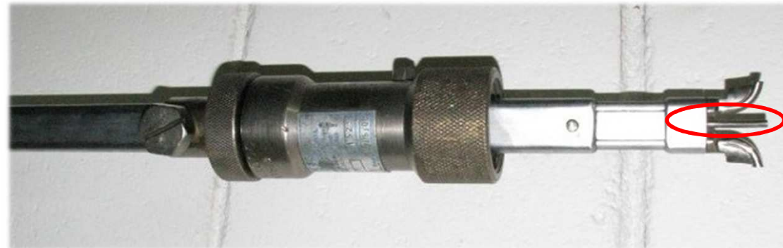
Modified Cole type Pitot tube with a safety pin in between the tips.
